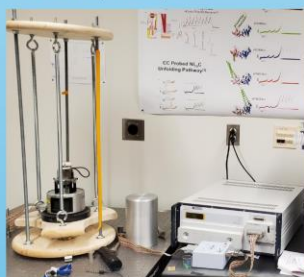
Scanning tunneling microscopy STM-based platform to investigate the putative interaction between tunneling electrons and odorants. Our STM vibration-isolation system is based on Dr. Dan Berard's design.
